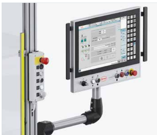
Optional CONTROL 3 multi-touch operating panel, free-standing, mounted on rollers or swiveling laterally on an arm, with display elements and control keys, visualization via 21.5" touchscreen
